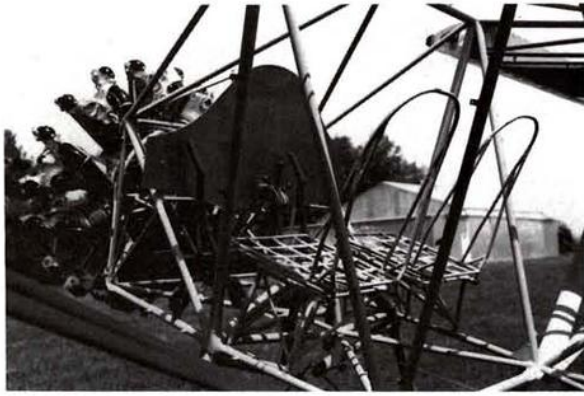
The instrument panel, cockpit controls and seats are in place.
